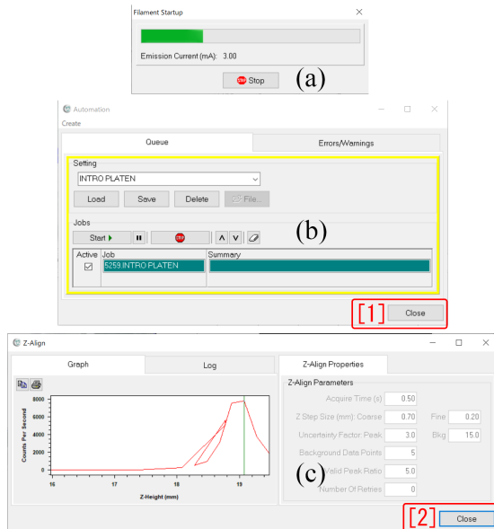
Figure 2.3: Window opened when starting the ‘Z-align’
