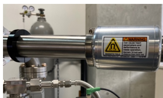
Figure 2.2: After V1 valve is opened, the sample introduction grip should be drawn such as to stop at ‘[1] Small stopper’ as shown in Fig. 1.11 (b)
