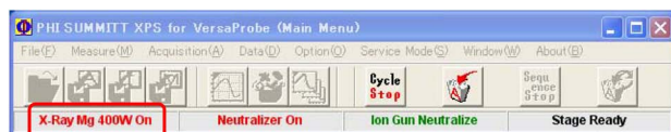
Figure A.4: In the main menu window indicating that Mg K\alpha X-ray source has been ON.
