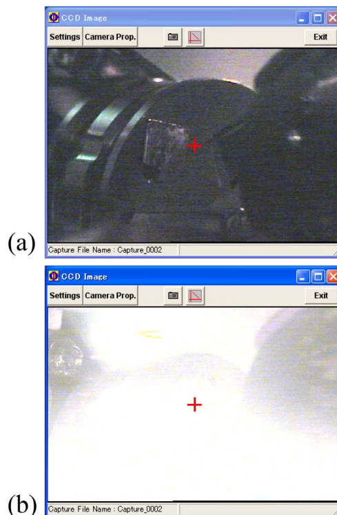
Figure A.5: (a) dark main chamber comes to be (b) bright by being illuminated by the filament when the Mg&Zr X-ray source is ON.
