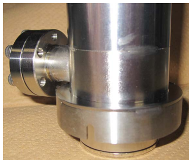
Figure B.3: The bottom of the transfer vessel has been closed.
