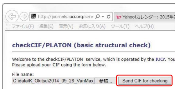
Figure 2.54: ‘Cif.cif’ is sent to IUCr web site by clicking ‘Send CIF for checking’ button.
