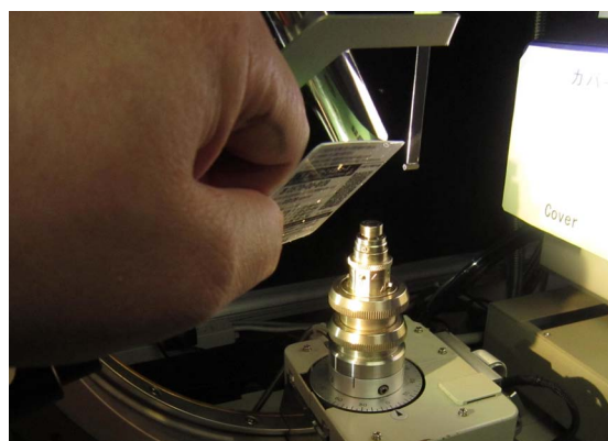
Figure 3.4: Mount of the crystal
