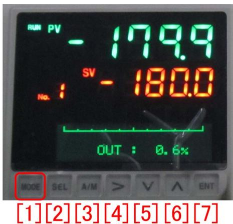
Figure A.1: Enlargement of the temperature setting unit in Fig. 1.1[p.1].
