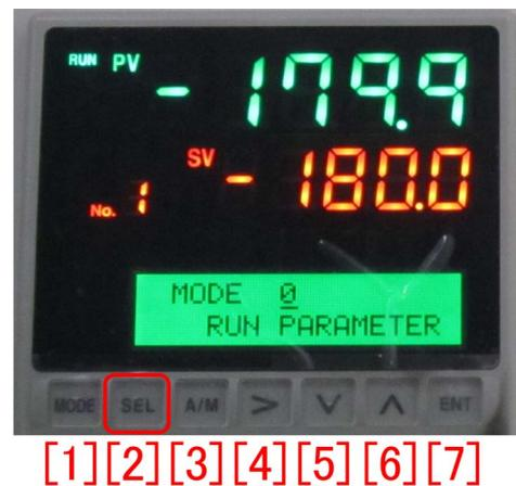
Figure A.2: '[1] [MODE] button' in Fig. A.1 has been pressed.
