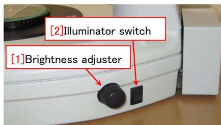
Figure B.2: Illuminator switch and brightness adjuster.
