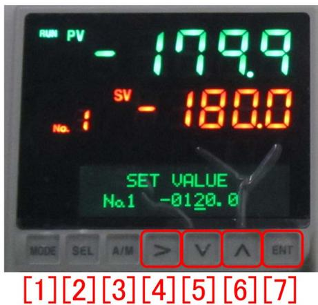
Figure A.3: ‘[2] [SEL] button’ in Fig. A.2 has been pressed to change the set temperature.
