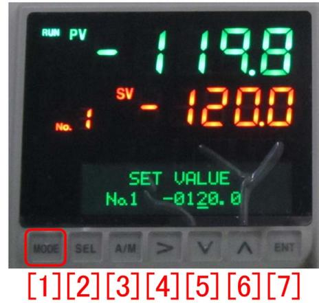
Figure A.4: ‘[7] [ENT] button’ has been pressed such that the temperature reaches to  $-120^{\circ}\text{C}$ .
