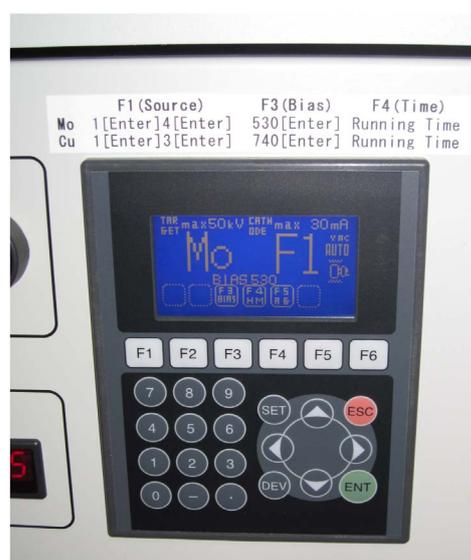
Figure 1.2: X-ray power setting panel
